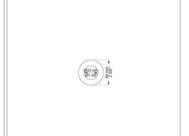
**001** 60 mm circular flange. Hole Ø33 mm.
