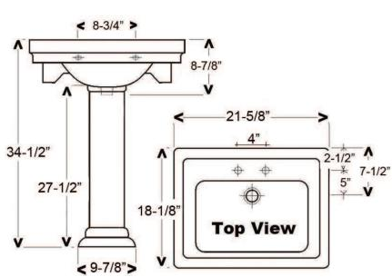
Basin Interior: 16" x 12" BasinDepth: 8" Mount bolts height: 32" Mount holes cc: 8 1/2" Faucet and spout holes: 1 1/8"(4") 1 3/8"(8")
