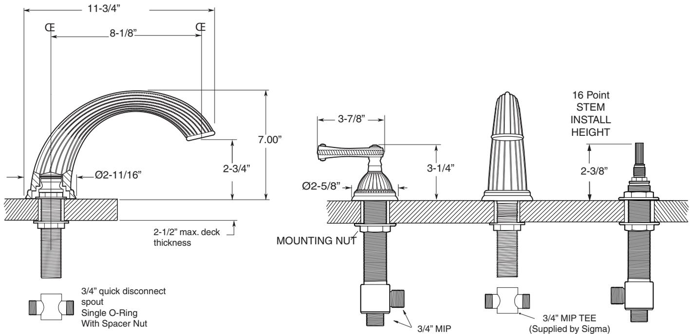
**NOTE:** Spout and valves install through 1-1/4" diameter holes. Plumber to provide 3/4" supply lines to valves
