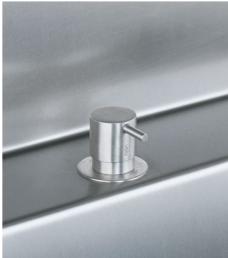
S50 Stop valve with 1/4 turn ceramic disc technology. Includes non-return valve and 1/2" inlet/outlet. Hole cut out size: 28 mm max 35 mm.
