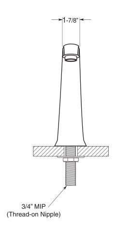
NOTE: Spouts install through 1-1/4" Diameter Holes.
