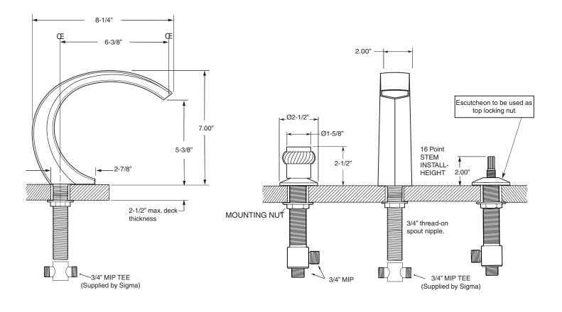
NOTE: Spout and valves install through 1-1/4" diameter holes. Plumber to provide 3/4" supply lines to valves
