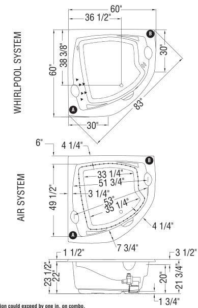
Note: A or B pump location could exceed by one in. on combo.
