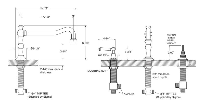
NOTE: Spout and valves install through 1-1/4" diameter holes.
