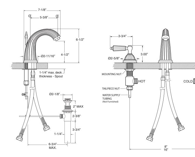
**NOTE:** Spout and valves install through 1-1/4" diameter holes
