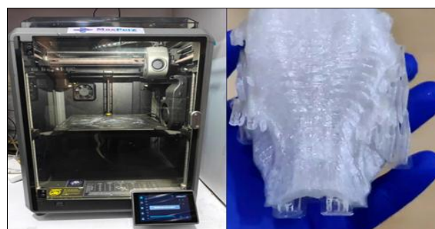
Fig 2: Left: In-house 3D printer used at MaxPetZ Hospitals to fabricate the patient-specific skull model. Right: 3D-printed anatomical skull model derived from CT DICOM data, used for preoperative landmark planning and craniotomy window simulation
