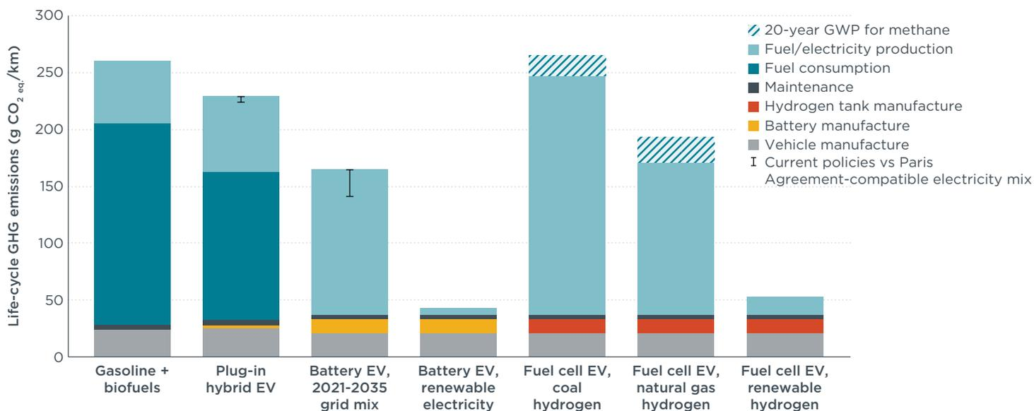
**Figure 5.2.** Life-cycle GHG emissions of A segment gasoline ICEVs, PHEVs, BEVs, and FCEVs registered in China in 2021.
