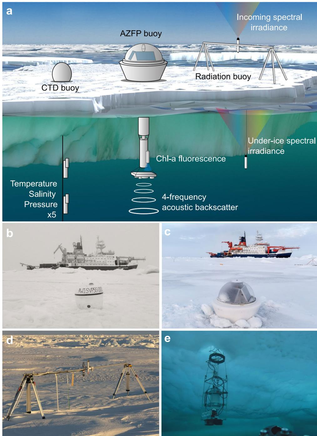
**Extended Data Fig. 1 | Autonomous bio-physical sea-ice observatory.** **a**, Schematic of drifting observatory; **b**, CTD buoy surface unit; **c**, AZFP buoy surface unit; **d**, Radiation station; **e**, AZFP buoy underwater package photographed by a remotely operated vehicle.
