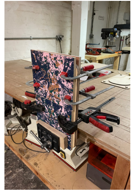
Laminating a plywood mould
