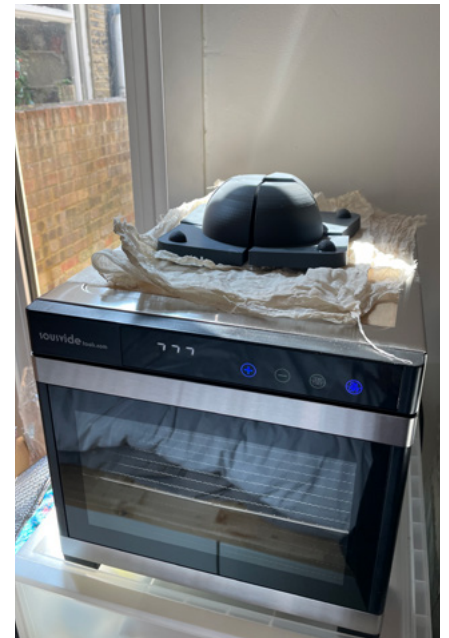
Testing durability of a PLA mould in the dehydrator
