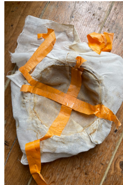
Cheesecloth as a de-moulding mechanism
