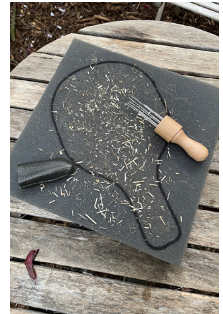
Tools for felting a sheet of flax, a borrowed process from wool felting
