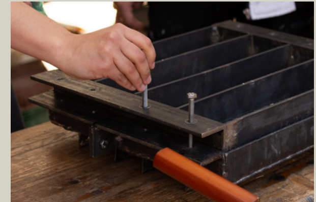
Development of a heavy metal press designed much like a flower press for mould pressing
