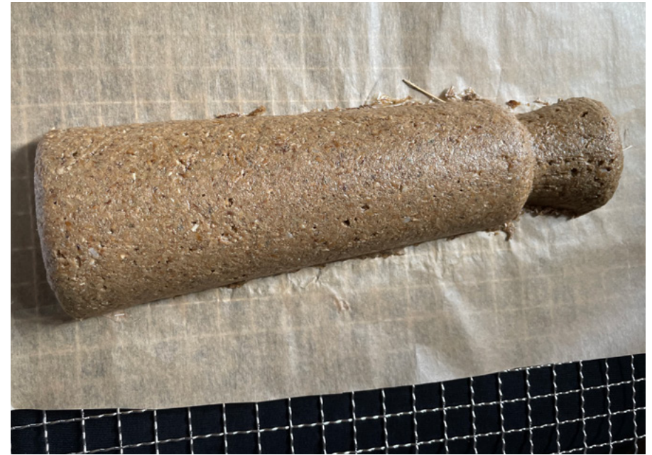
Half a skittle cast from plaster
