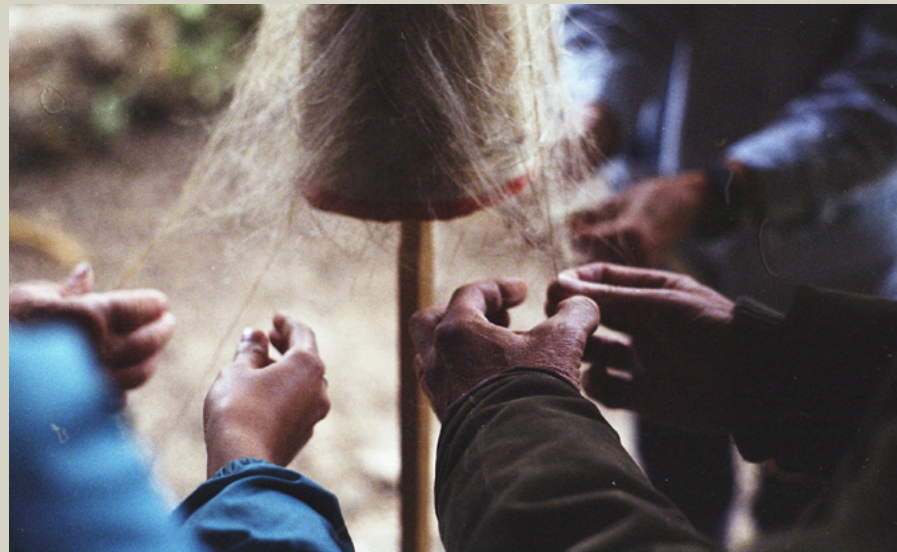
Spinning flax fibre on a cone distaff
