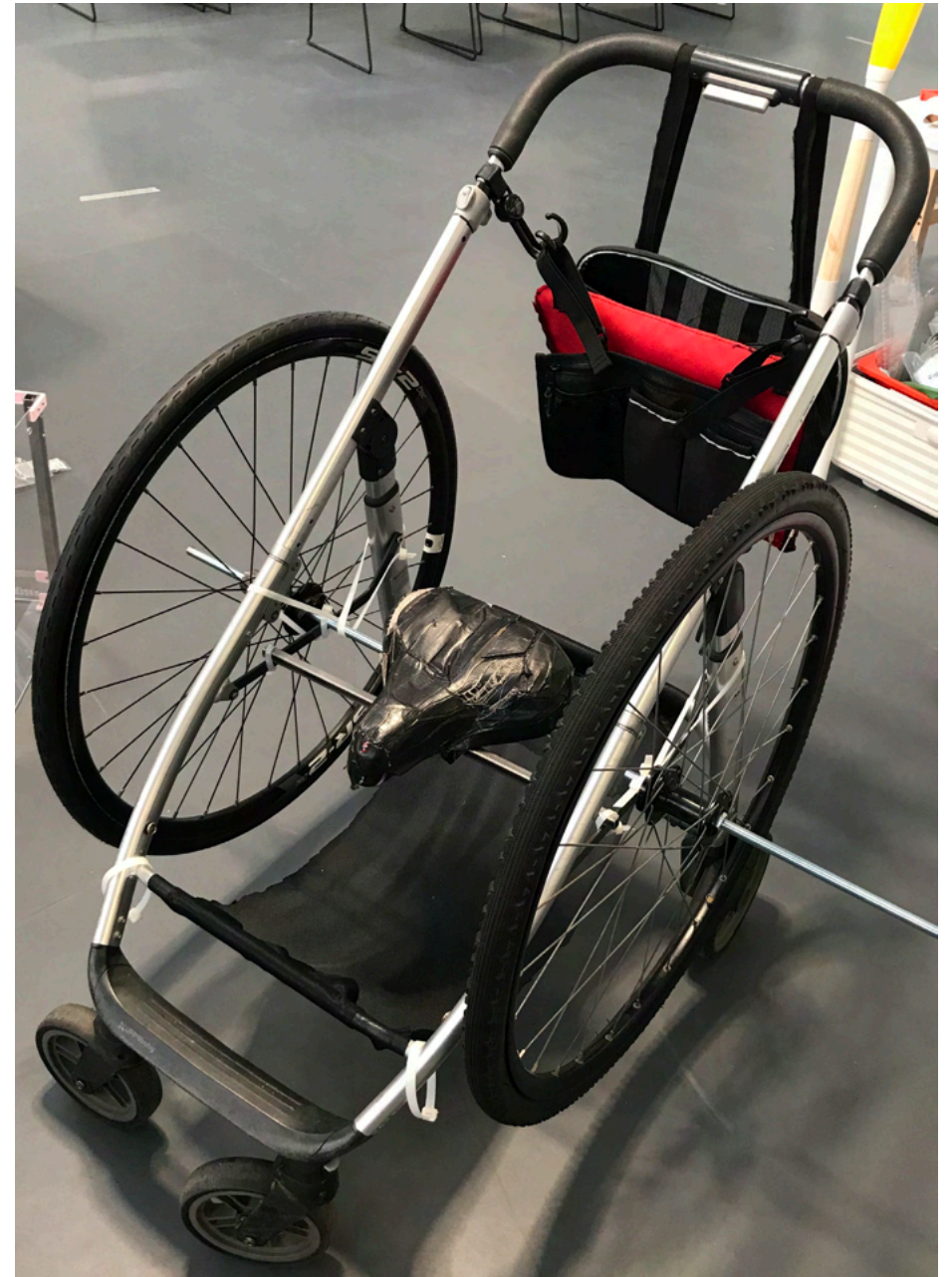
TESTING WITH ACTUAL BIKE SEAT, WITH NEW SYSTEM OF ATTACHING THE BIKE WHEELS AND SEAT
