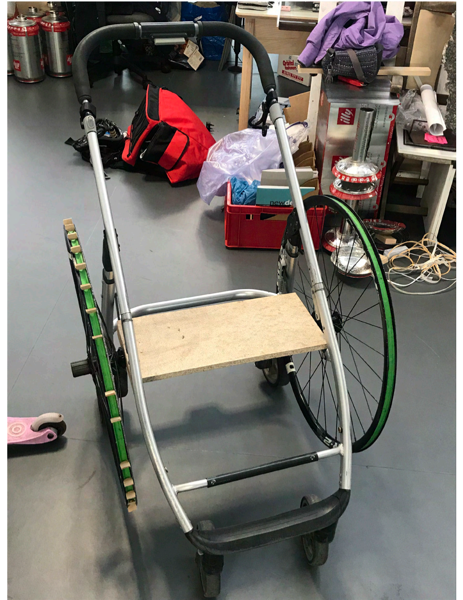
TESTING OF SEAT PLACEMENT AND WEIGHT SUPPORT INITIAL INSTALLATION OF WHEELS
