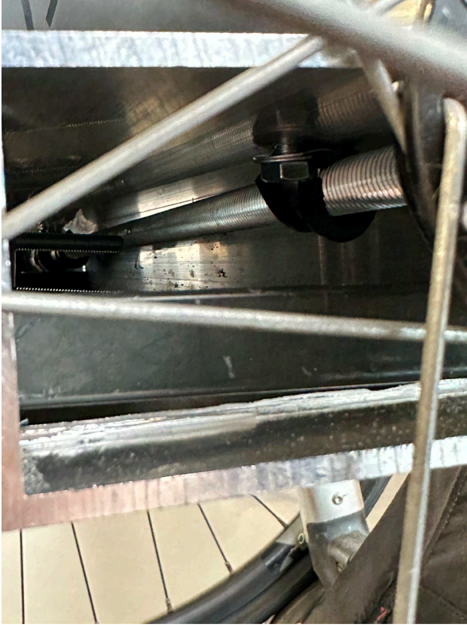
THE THREADED STEEL ROD THAT GOES THROUGH THE BOX SECTION IS SECURED WITH 2 RUBBER LINED CLAMPS, WITH ONE BIKE WHEEL ATTACHED ON EACH END
