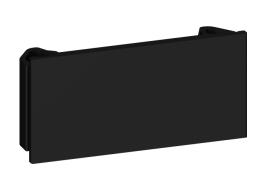
The blind cover is used as protection against accidental contact for standard-compliant sealing of unused ports of screens for 3-pole industrial connectors or is also used only as dust protection. As a result of the standardized dimensions, it is suitable for simple and flat snap-in mounting flush with various U-Box screens with industrial connector cut-outs.
