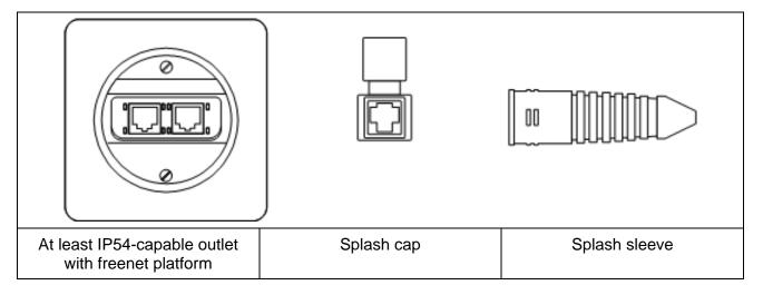
Protection class IP54 is also high enough to protect connecting hardware against dust and moisture in outdoor applications.
