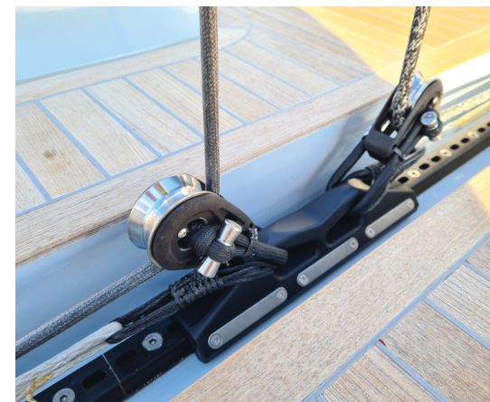
Above: Rigging Projects' new X Car on the mainsheet track of the Mills 68, Pelotari. Left: Rigging Projects' jib halyard locks now have integrated load cells. Above right: North Sails' Design Suite software enabled the Gunboat 80 rig design team to fast-track load results and hardware placement
