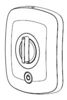
It is necessary to engage the control knob on the correct position on the valve spindle before the front cover is located.
