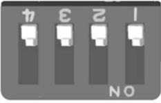
On the main Logic PCB : Set the red DIP switch N° 1 to the Off position.
