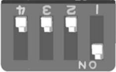
On the main Logic PCB : Set the red DIP switch N° 1 to the ON position.
