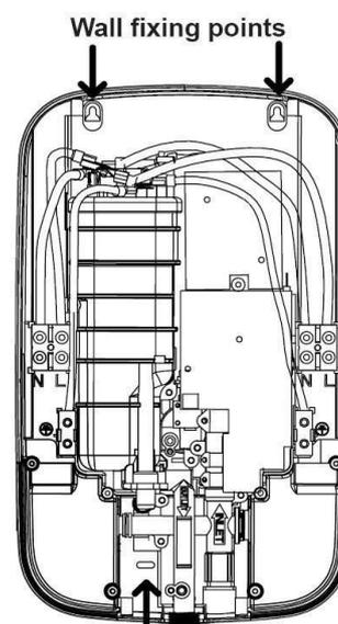
**NOTE:** The bottom screw should only be fitted during final installation.
