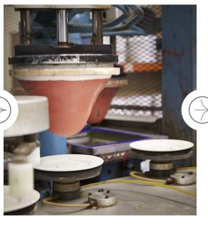
The vast majority of our flat items such as plates and bowls are decorated by machine using the underglaze printing process. This involves a silica bomb, an engraving and thermoplastic colours. Colour is spread onto the engraving; the silica bomb takes an imprint of the pattern and transfers it to the plate. We are able to print up to 4 colours on one machine in this way and to an exceptionally high standard.
