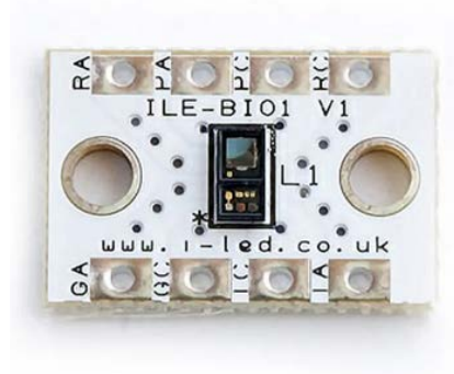
Fig. 22. The BIOFY Eco1 SFH 7050 board has mounting holes for M3 screws and has dimensions of 20.25mm x 13.7mm x 0.9mm. (Image: RS Components)
