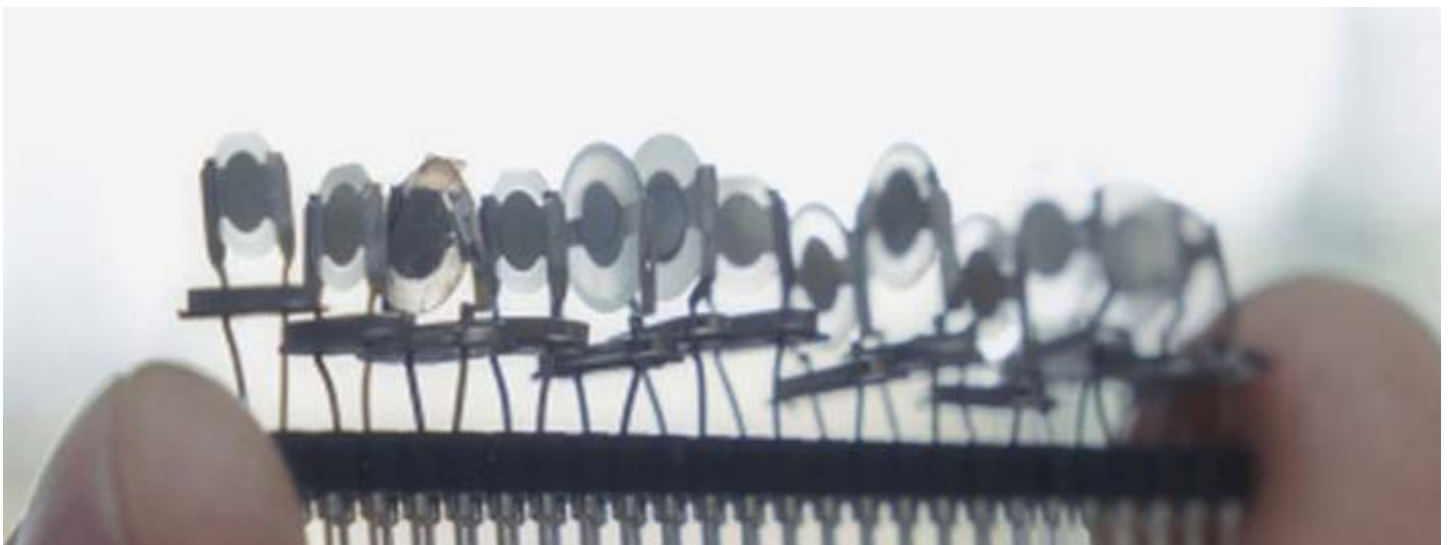
Fig. 14. It doesn't look like a nose at all: a combination of sensors and materials enables the artificial sense of smell. (Photo: Press photo Amadeus Bramsiepe, KIT)
