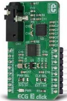
Fig. 4. The click board is suitable for use on a system with a microbus connection and is used for prototyping. (Image: RS Components)
