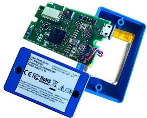
Fig. 12. In addition to many other functions, the STEVAL-MKSBOX1V1 from STMicroelectronics can be used to implement a pedometer (Image: RS Components)
