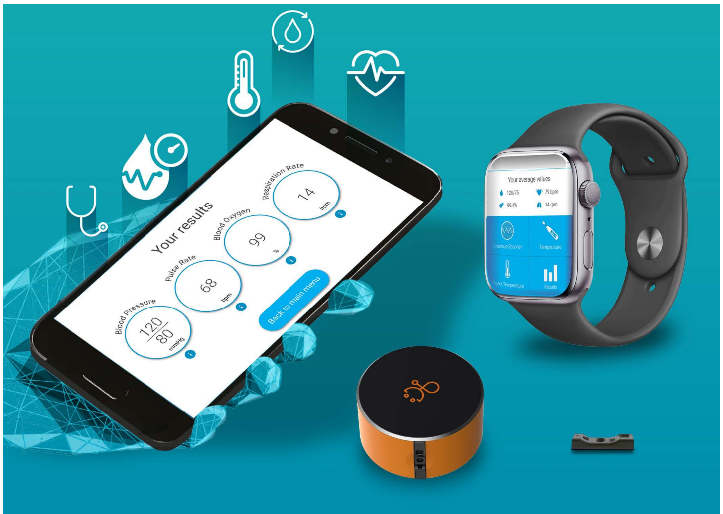
Fig. 4. A stand-alone miniature V-sensor device from Leman Micro Devices sends the measurement results via Bluetooth to a smartphone. There, the e-Checkup app shows the results of the blood pressure measurement. (Image: Press image Leman Micro Devices)
