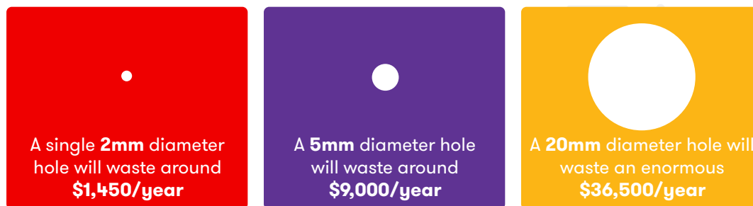
Fig 1: Approximate cost of an individual air leak
