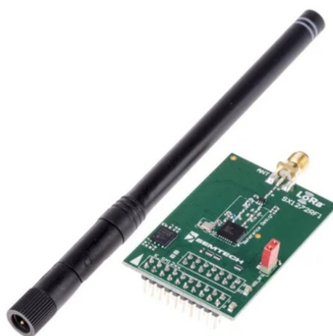
Fig. 4. 868-MHz-ISM-Band-Transceiver-Evaluation Module from Semtech with LoRa technology. (Image: RS)
