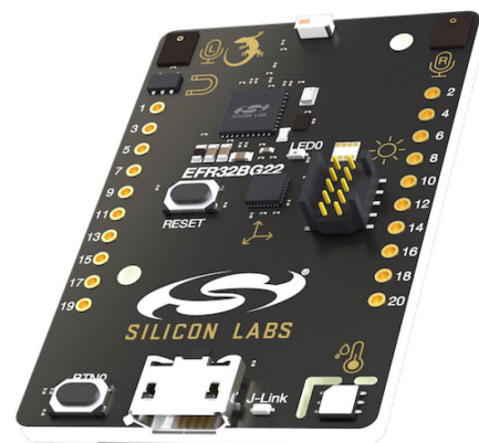
Fig. 7. The EFR32BG22 module is used in the Silicon Labs Bluetooth Direction Finding solution. (Image: Press image Silicon Labs)
