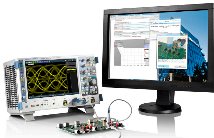
Fig. 3. With the K58 option for the R&S RTO and R&S RTP oscilloscopes, tests can be carried out for 1000BASE-T1 Single Pair Ethernet. (Image: Rohde & Schwarz)
