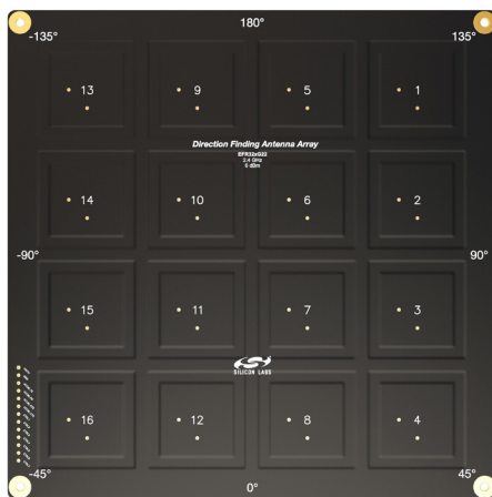
Fig. 6. Silicon Labs Direction Finding Antenna Array, der benyttes i Bluetooth Direction Finding-løsningen fra SiLabs. (Billede: Pressebillede Silicon Labs)
