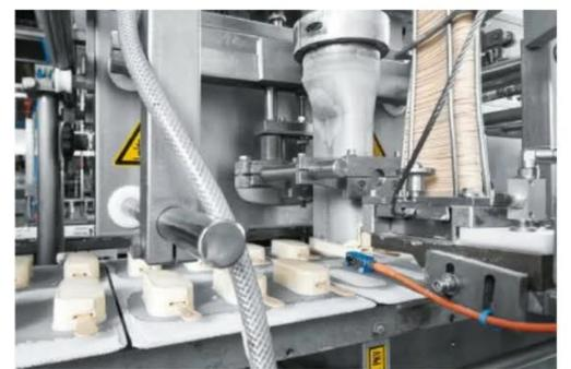
**Perfect portions:** The extruder outputs one Magnum core per second. The stick is inserted in the ice cream during extrusion.
