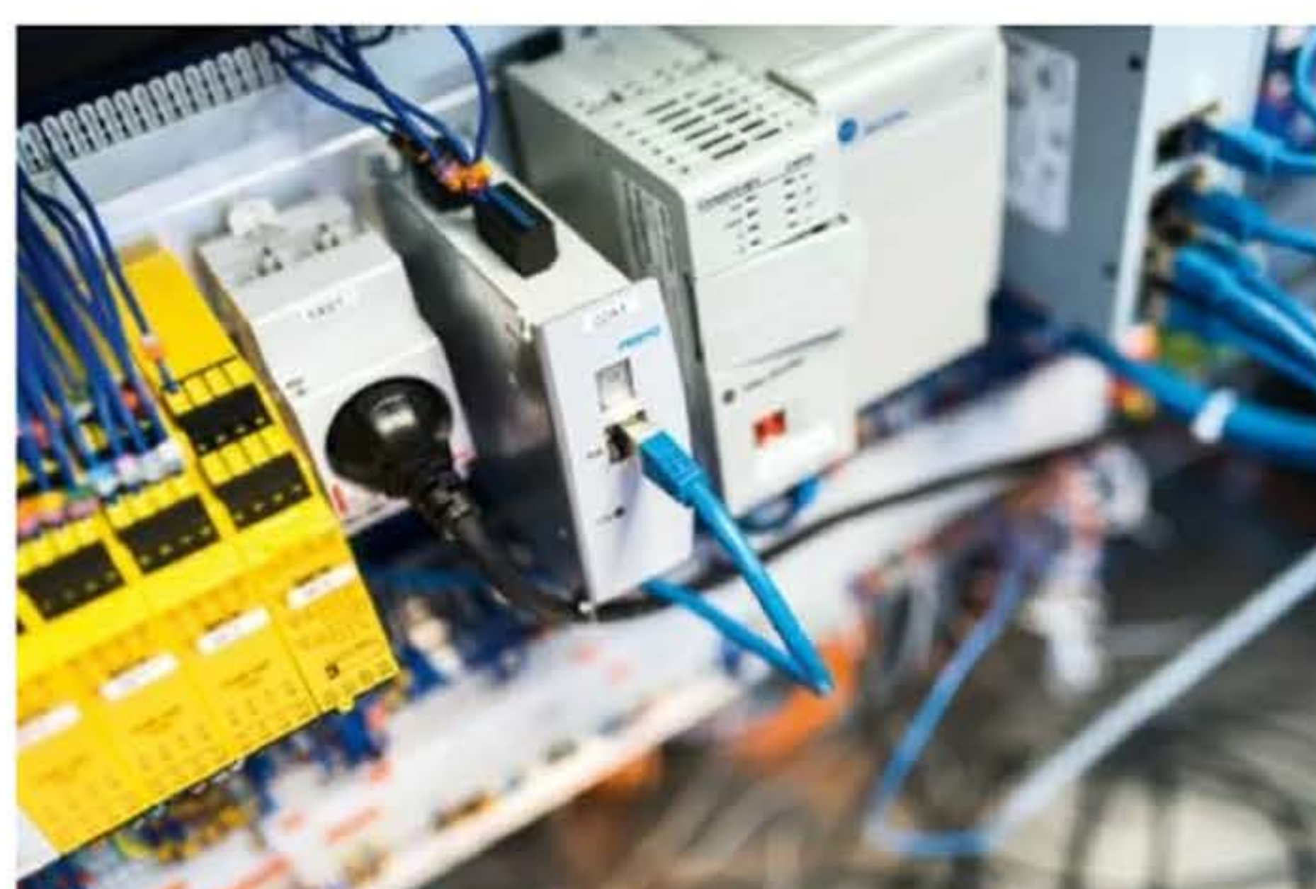
Small but beautiful: The controller CMMO controls the electric cylinder EPCO, connected via IO-Link®.
