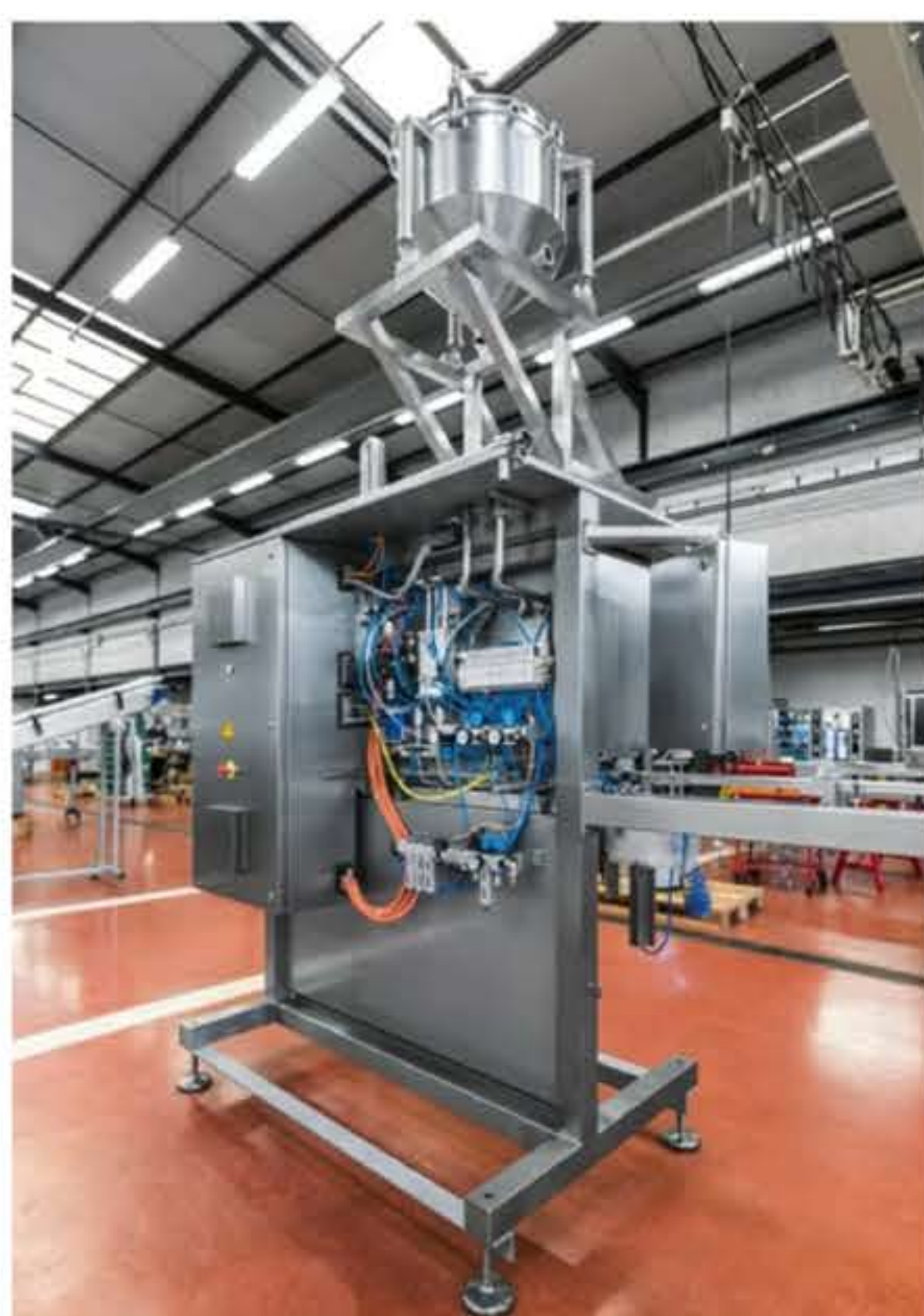
Still in the assembly process: SF102—filling and sealing system for Doypack® pouches with screw cap.
