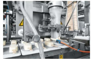
Perfect portions: The extruder outputs one Magnum core core per second. The stick is inserted in the ice cream during extrusion.
