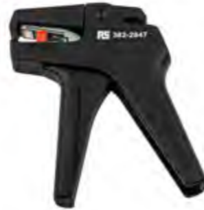
382-2847 0.08 to 2.5mm stripping range 384-7385 6 to 16mm stripping range
