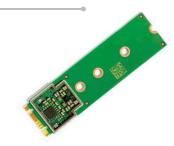
The Google coral M.2 accelerator is an M.2 module that brings the edge TPU coprocessor to existing system and products. It enables easy integration into ARM and x86 platforms so it can add local ML acceleration to product such as embedded platforms, mini-PCs, and industrial gateway. It's weight is
