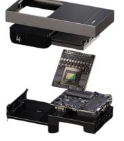
The NVIDIA® Jetson AGX Thor™ Developer Kit is the ultimate platform for humanoid robotics, giving you unmatched performance and scalability. It's powered by the NVIDIA Blackwell GPU and 128 GB of memory, delivering up to 2070 FP4 TFLOPS of AI compute to effortlessly run the latest generative AI models-all within a 130 W power envelope. Compared to NVIDIA Jetson AGX Orin™, it provides up to 7.5x higher AI compute and 3.5x better energy efficiency.
