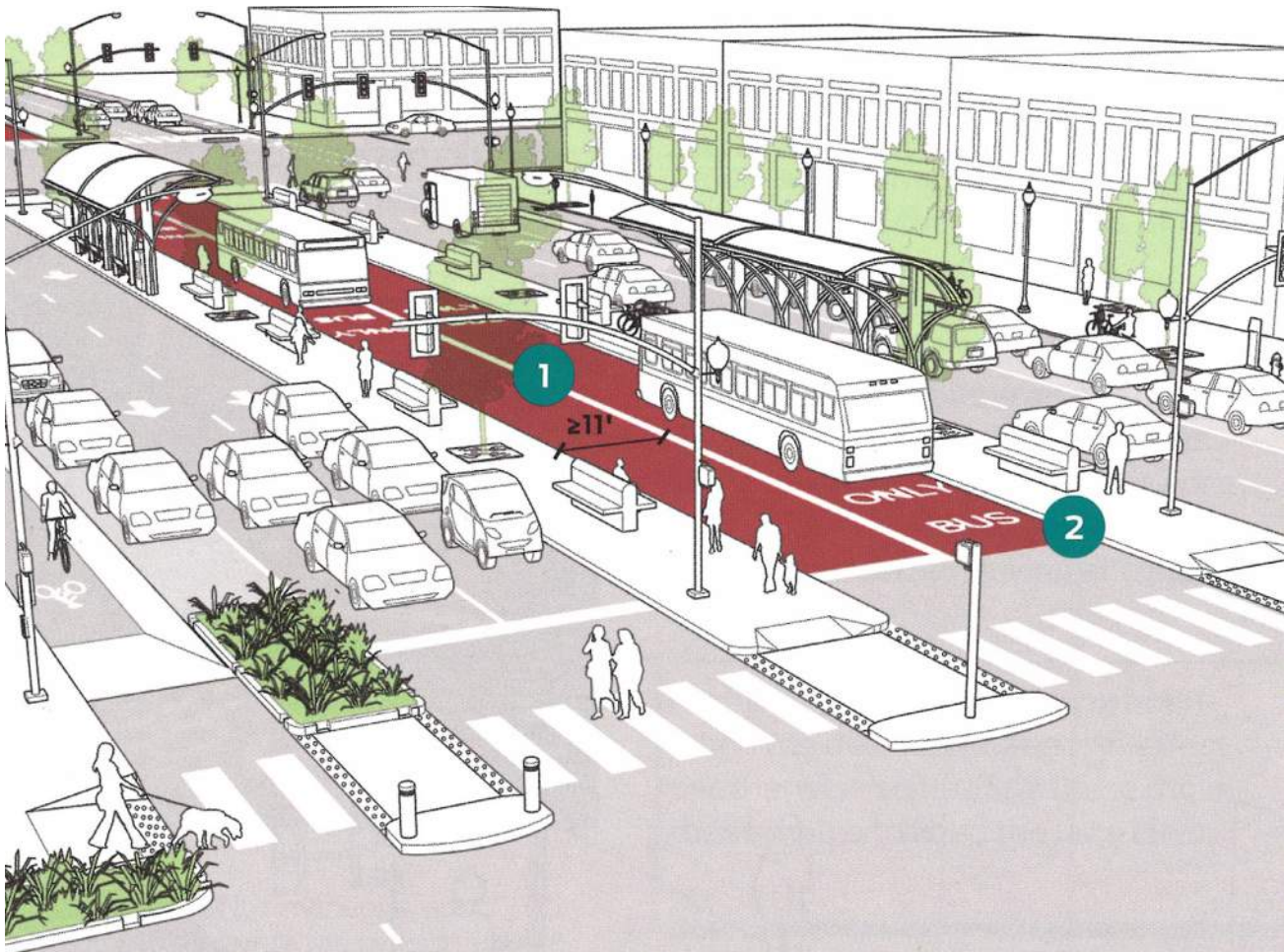
Major Transit corridor prototype (Source: National Association of City Transportation Officials Urban Street Design Guide )
