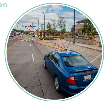
Accelerate testing of bicycle/pedestrian detection at crossings
