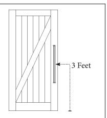
The center point of the door pull should be three feet above the bottom edge of the door. Avoid placing the door pull too close to the edge of the door. Placing the pull too close to the edge can damage both door and pull.
