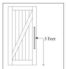
The center point of the door pull should be three feet above the bottom edge of the door. Avoid placing the door pull too close to the edge of the door. Placing the pull too close to the edge can damage both door and pull.
