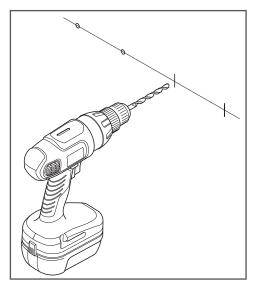
6. Drill out the marked holes using a drill with a 1/4" drill bit (Figure 3).
