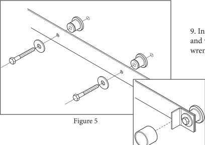
9. Install remaining spacers with lag screws and washers (provided) using a 9/16" socket wrench (Figure 5). Tighten all lag screws.
