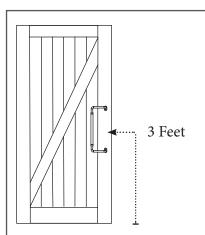
The center point of the door pull should be three feet above the bottom edge of the door. Avoid placing the door pull too close to the edge of the door. Placing the pull too close to the edge can damage both door and pull.
