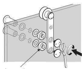
Remove the spacer when used with 1-3/4" wood door.
