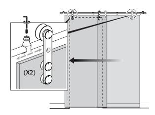
9. Re-attach anti-rise pin into hangers.
