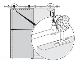
9. Re-attach anti-rise pin into hangers.
