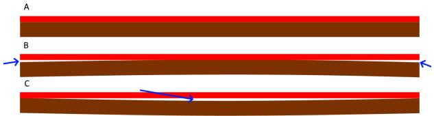
This same process should be used on the side of the door (the narrow edge). Using the straight edge on the front (or back) of the door and on the side (edge) of the door should be all the measurements needed. You can also lay the straight edge "corner to corner" diagonally across the door.
