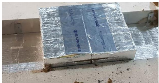
Fig 5 Stubguard® fitted for testing at Warringtonfire
