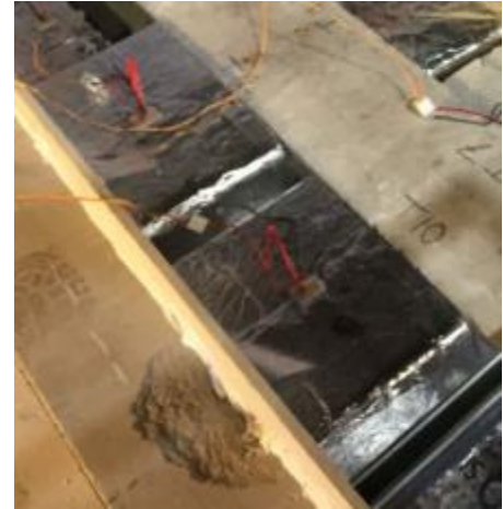
Fig 2 Stubguard® testing at Warringtonfire. Note sensors monitoring top surface temp.
