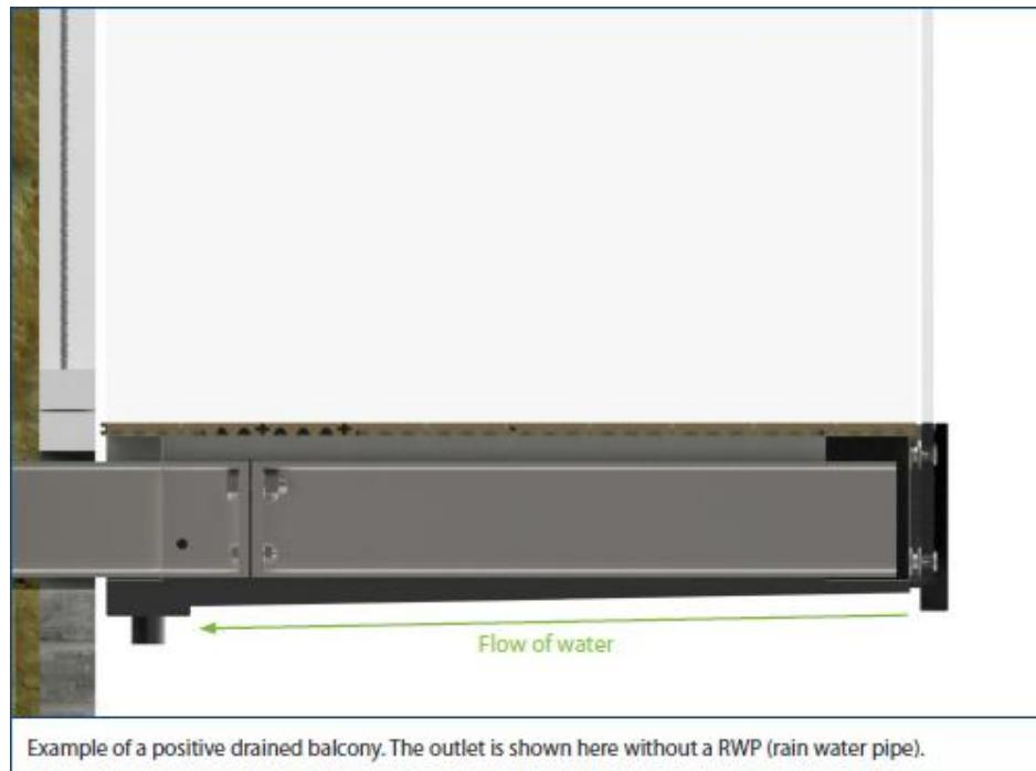
Water is directed towards the back of the balcony into rainwater pipes running down the building façade.
