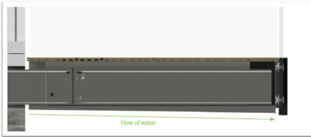
Balcony soffits have a gradient, usually sloped to the front of the balcony, so that rainwater will flow towards the front of the balcony, where it can freely drain. This effectively channels the water away from the building façade without the need for pipes.
