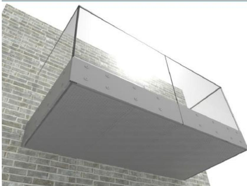
Water is either drained through the gaps between the decking, without any form of water management. Or, are free draining balconies using soffits with perforations. The use of perforated soffits offers balconies a neater aesthetic appearance than not using soffits as it hides the balcony supports and their connections.
