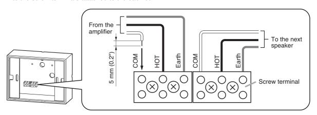
3-2. Insert the fasten s fitted at the ends of the HOT and COM cables from the screw terminals on the cabinet into the taps of the matching transformer on the speaker unit. Connect the COM cable to the transformer's COM tap, and the HOT cable to the desired transformer's input tap (Refer to the figure at right.)
