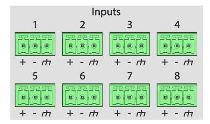
Connect input AV devices to the 3-pin inputs.
