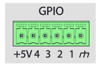
These GPIO connections can be used as either inputs or outputs. They can be assigned to actions within Tesira software using Logic Input and Logic Output.
