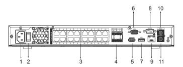
Power Switch 1 Power Input PoE Ports Alarm In/Out 3 HDMI Port VGA Port 5 6 USB Port RS-232 Port 7 8 Network Port AUDIO OUT, RCA Connector 9
