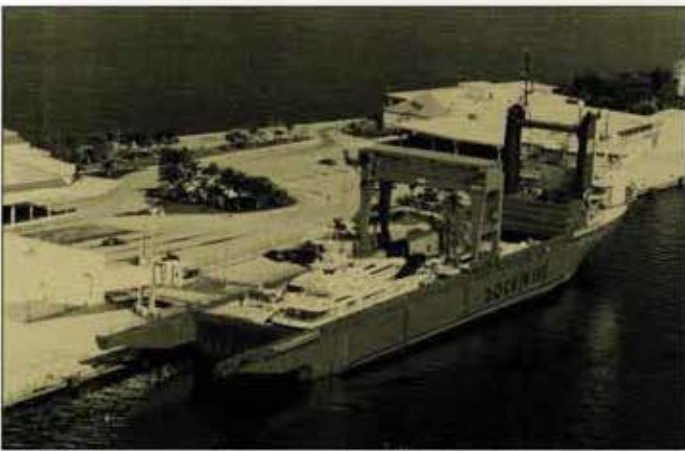
1989: Dock Express begins unique float-on/float-off (flo/flo) service using vessels with submersible hulls to ship yachts overseas. In '92, the firm becomes United Yacht Transport and in the new century, Dockwise Yacht Transport.
