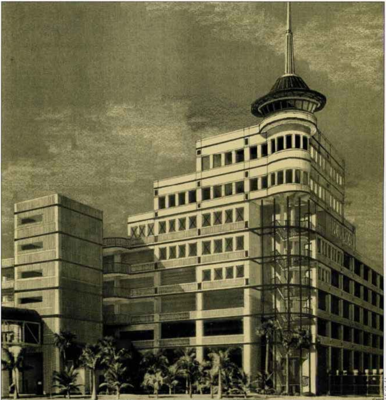
1999: Rendering depicts expansion of the Midport Parking Garage, being doubled from 1,000 parking spaces to 2,000 and dominated by a Operations/Harbormaster Tower standing nearly 110 feet tall. Construction begins in '99 with completion anticipated summer 2000.
