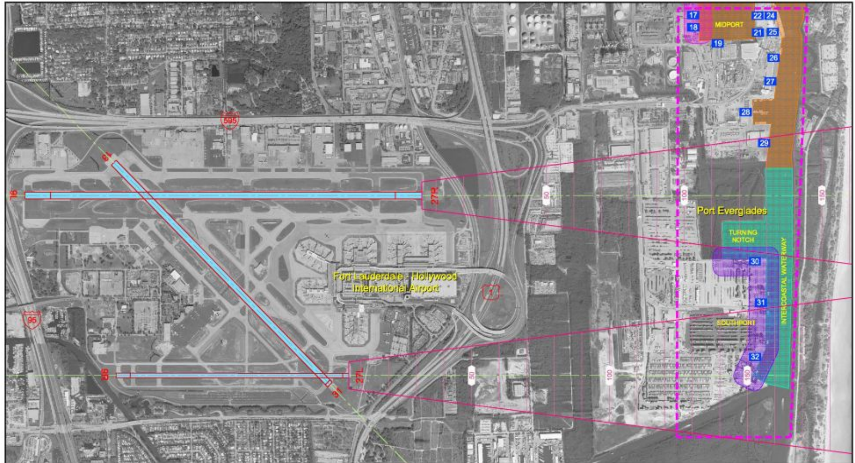
Figure 7 ICAO ONE ENGINE INOPERATIVE (OEI) SURFACE OVER STUDY AREA EXISTING CONDITIONS Airspace Obstruction Study Port Everglades Cranes and Ships Fort Lauderdale-Hollywood International Airport November 2008
