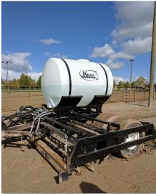
The Equestrian Park crew is pleased to add a new piece of equipment to enhance arena prep. The Kiser (left), which grooms and waters the footing, is being used primarily in the indoor and covered arenas.
