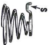
Fig. 25. Stop Washer and Tension Spring
