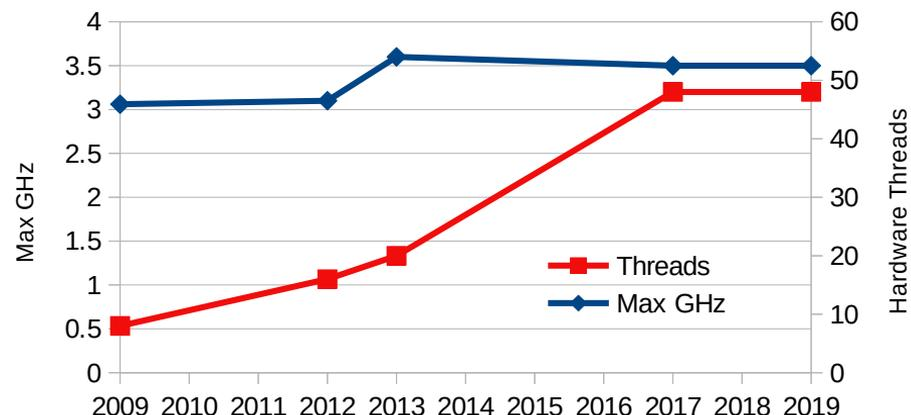
Increase has leveled off due to power/efficiency
